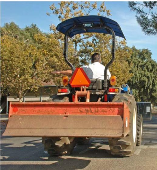
That fluorescent orange triangle you usually see on the back of tractors, implements, forklifts, and other equipment on public roads is called a Slow Moving Vehicle or SMV emblem. It is intended to alert drivers of following vehicles to slow down for the SMV-signed vehicle in front that is travelling at 25 mph or much less. Tractors and forklifts typically may be going only 5 to 15 mph, presenting a real hazard on roads where other traffic may be going up to 55 mph.
