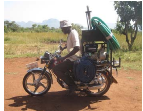
Completed Mobile Irrigation System, ready to roll.
